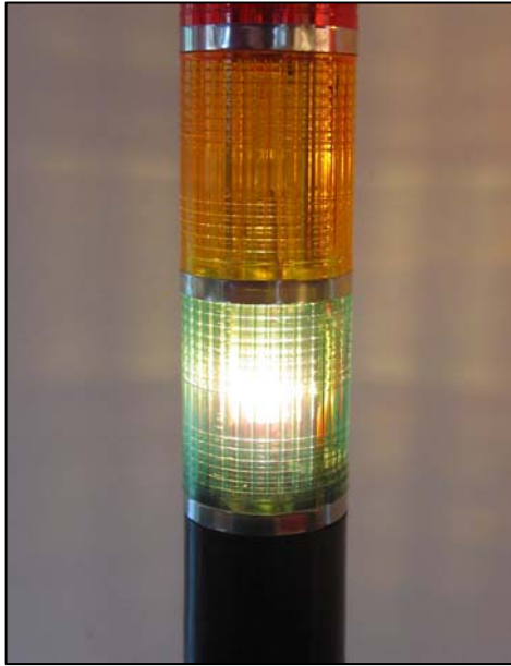
Figure 7 The green light is lit after sending the G character
